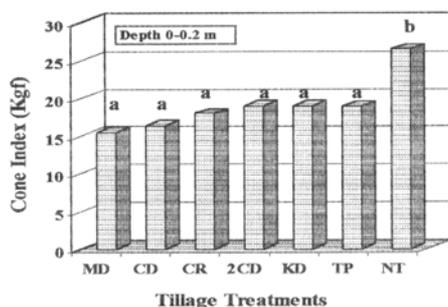
**Figure 1.** Cone index (CI) taken in seven tillage systems (means of 10 points) at 0-0.1 and 0-0.2 m layers. Means with the same letter are not significantly different ( $P < 0.05$ ). DM= moldboard + disk, CD= chisel + disk, CR= chisel + rotary, 2CD= chisel (twice) + disk, KD= khishchi, TP= till planting with cultivator combined drill, NT= no-tillage.
