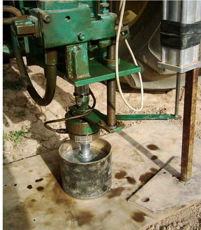
Fig. 4. In situ confined compression test
