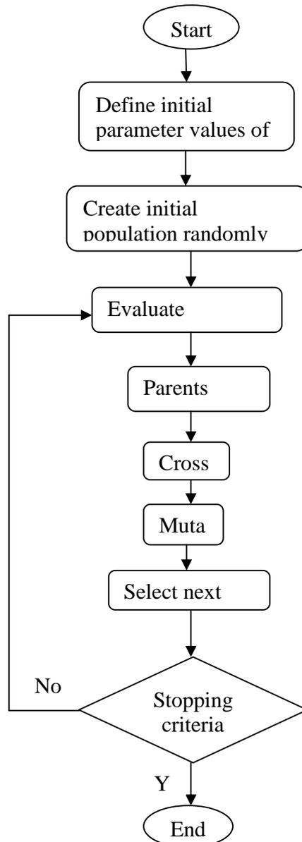
Figure 1. Blocky diagram of a real genetic algorithm
