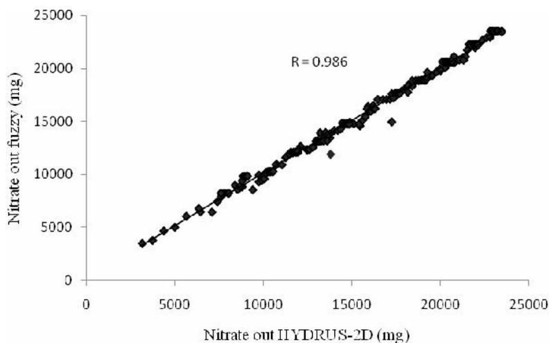
Figure 4. Estimates of cumulative nitrate leaching during entire growing season by the MFIS model using training data versus outputs from HYDRUS-2D
