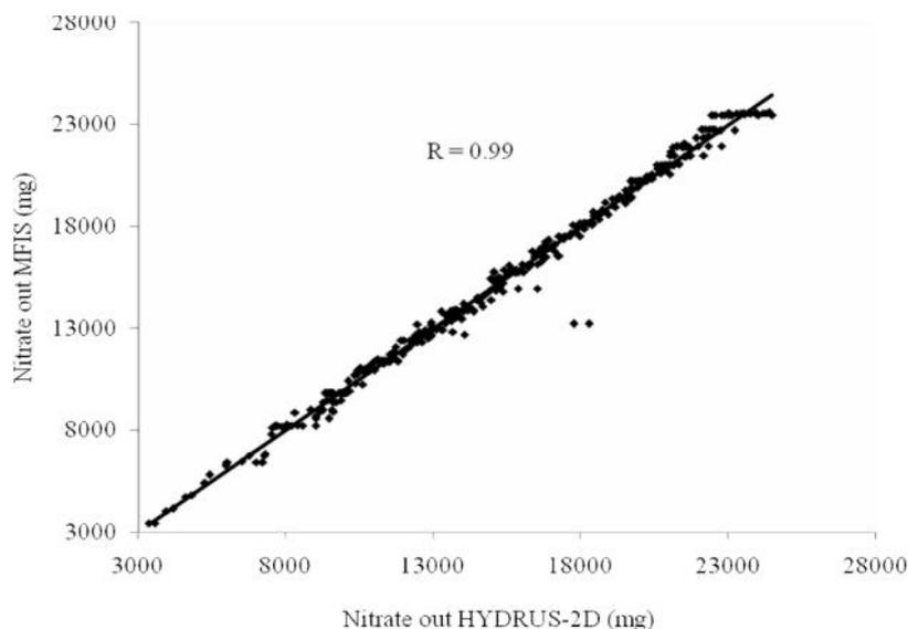
Figure 5 Estimates of cumulative nitrate leaching during entire growing season by the MFIS model using test data versus outputs from HYDRUS-2D.
