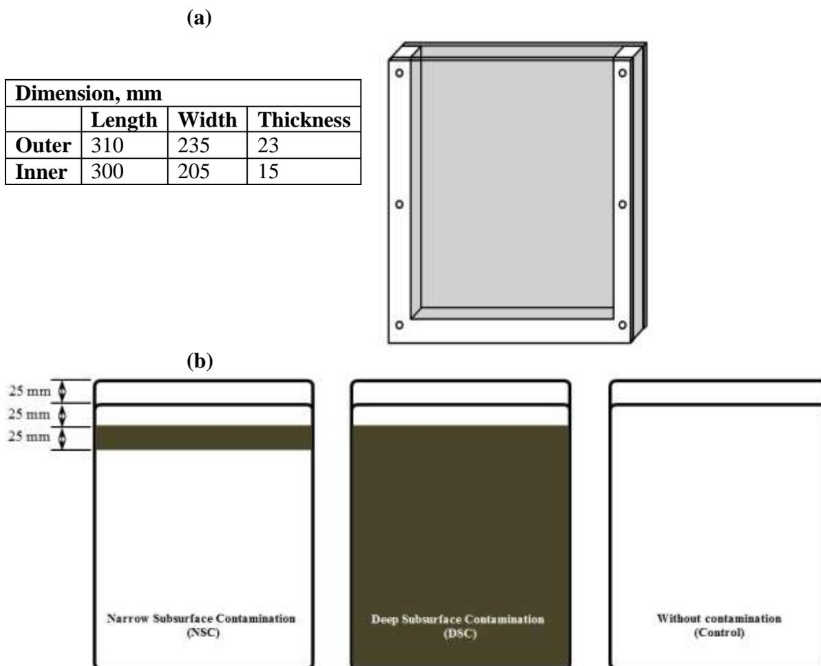
**Fig. 1.** Rhizotron dimensions (a) and applied soil contamination patterns (b).
