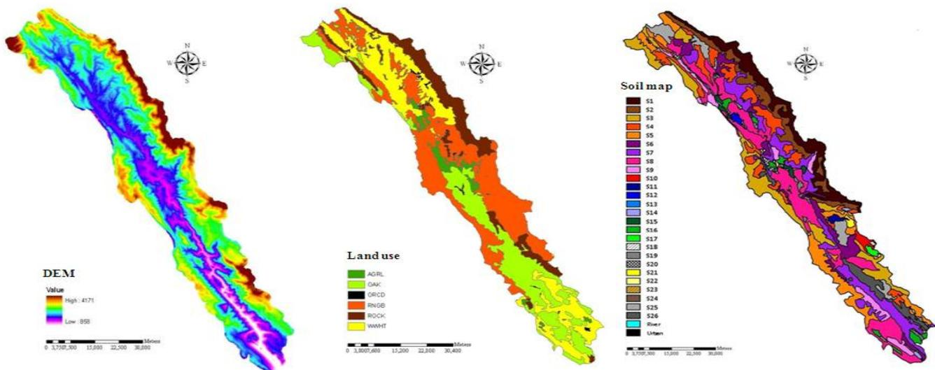
Fig. 2. The input maps to SWAT (DEM: digital elevation model, landuse, and soil maps)
