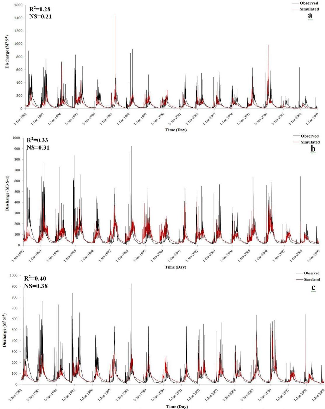
Fig. 3. Daily runoff prediction using SWAT models developed by different input climate data sets (a: CRU, b: CDW, and c: COM). R<sup>2</sup>: coefficient of determination and NS: Nash-Sutcliff coefficient.
